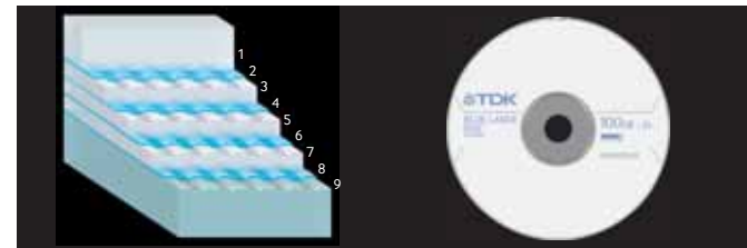
1 Cover layer 2 Recording layer (L3) 3 Spacer layer 4 Recording layer (L2) 5 Spacer layer 6 Recording layer (L1) 7 Spacer layer 8 Recording layer (L0) 9 Disc substrate
