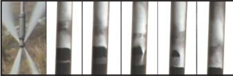
Unplugging jets penetrate, surround plugs, and grind away
