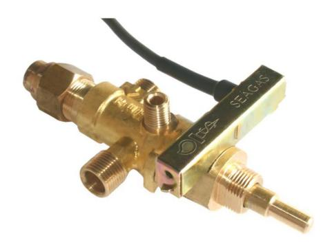
A combined taper plug valve and FSD control, available either with or without integral piezo. The range of spindle options, thermocouple connections and lengths of Ignitor lead has made this a popular valve in the decorative fuel effect fire market for many years.
