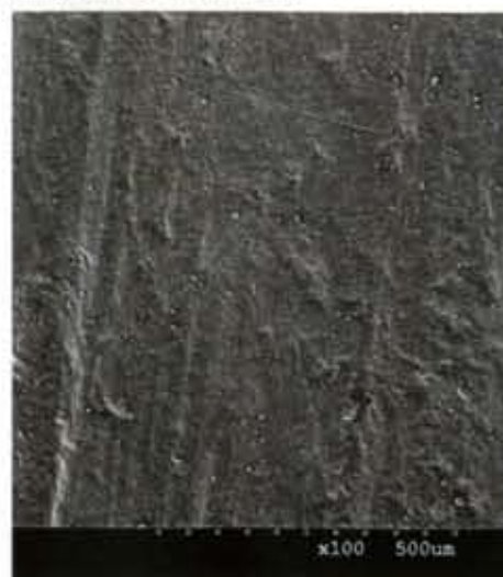
Below: FIG 2b – SEM image of microwear on a cast made from a GC Exafast mould
